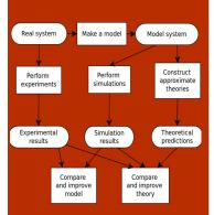
Process of building a computer model and the interplay between experiment, simulation, and theory
